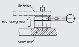
Make sure that no force on the underside of the workpiece exceeds the values given in the table.
